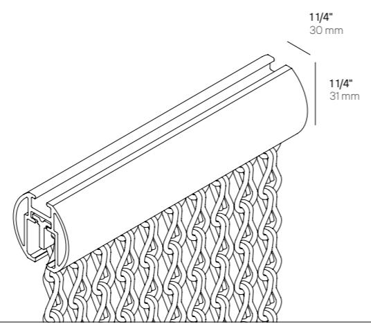
Tubular rail suitable for both straight and curved shapes.
