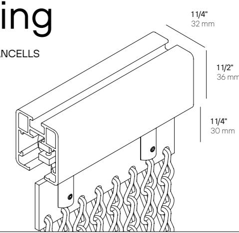
Movable rail system with slide rails that allow a 'panel' effect.
